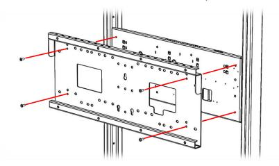
13. Attach the hangers to the back of the screen.
