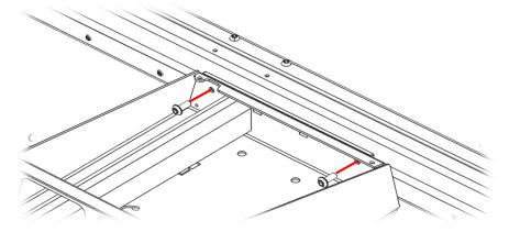
5. Plug the power cable into the transformer though the grommet indicated and bolt the rear panel in place.
