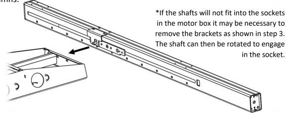
3. Gently remove the transportation brackets from columns as shown, put the bolts removed to aside for use later in the assembly process.
