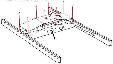
6. Attach the handle using the bolts you put aside in step 3 and the bolts already fitted in column. Use the top set of holes. Add the 16 caps into the holes indicated by the red arrows.
