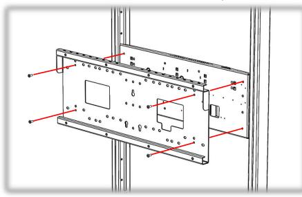
9. Attach the hangers to the back of the screen, make sure the hangers are
