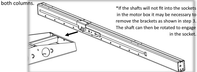
3. Gently remove the transportation brackets from columns as shown, put the bolts removed to aside for use later in the assembly process.
