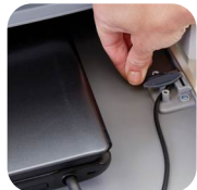
Twisting cable clips to keep devices in place and free from damage.
