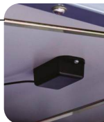
Built-in heat sensor will shut off power if a device overheats.
