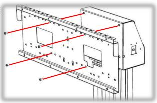
5. Atach the brackets to the back of the screen, make sure the brackets are as
