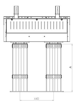
2. With the four brackets fixed to the wall move the heavy dduty li up to the brackets and check the alignment of the brackets with the columns. If the columns align with the brackets use the U-Shaped straps to secure the lif to the wall as shown in the diagram. Each strap should be secured with four M8 bolts.
