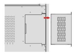
**Step 2** Slide the OPS into the OPS port on the rear of the panel until firmly seated.
