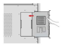
**Step 3** Secure the OPS to the display by using the M3 screws.
